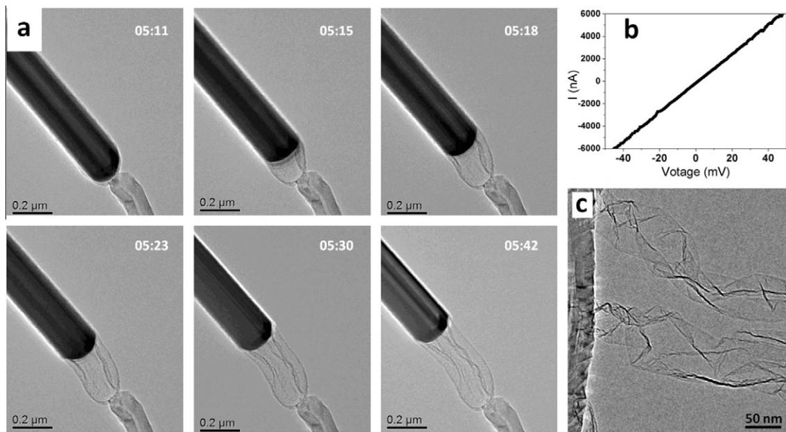
**Fig. 5 – (a)** An image sequence of extraction of a Ag nanowire by Joule heating under a large bias. The upper electrode is a Ag nanowire covered by amorphous carbon shell while the lower electrode is a commercial MWCNT adhered on a tungsten tip. **(b)** A measured I-V curve of the formed graphitized CTS in (a). **(c)** Graphene/graphite sheets formed by extraction of a Ag nanowire covered with thin amorphous carbon sheath under a large bias.
