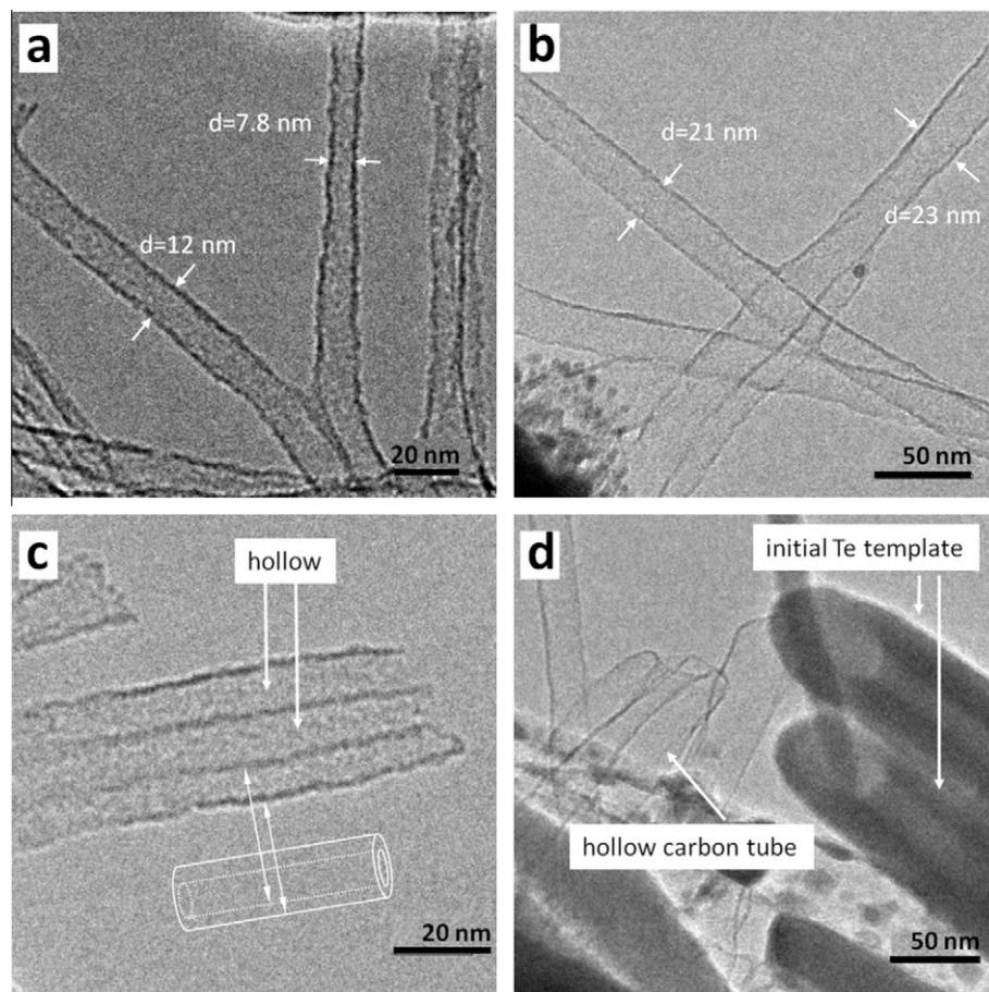
**Fig. 3 – Formation of thin CTSs with Te nanowires/nanotubes as templates. The diameters of the fabricated CTSs are around ten nanometers in (a) and twenty nanometers in (b). (c-d) Fabricated tube-in-tube CTSs with Te nanotubes as templates.**
