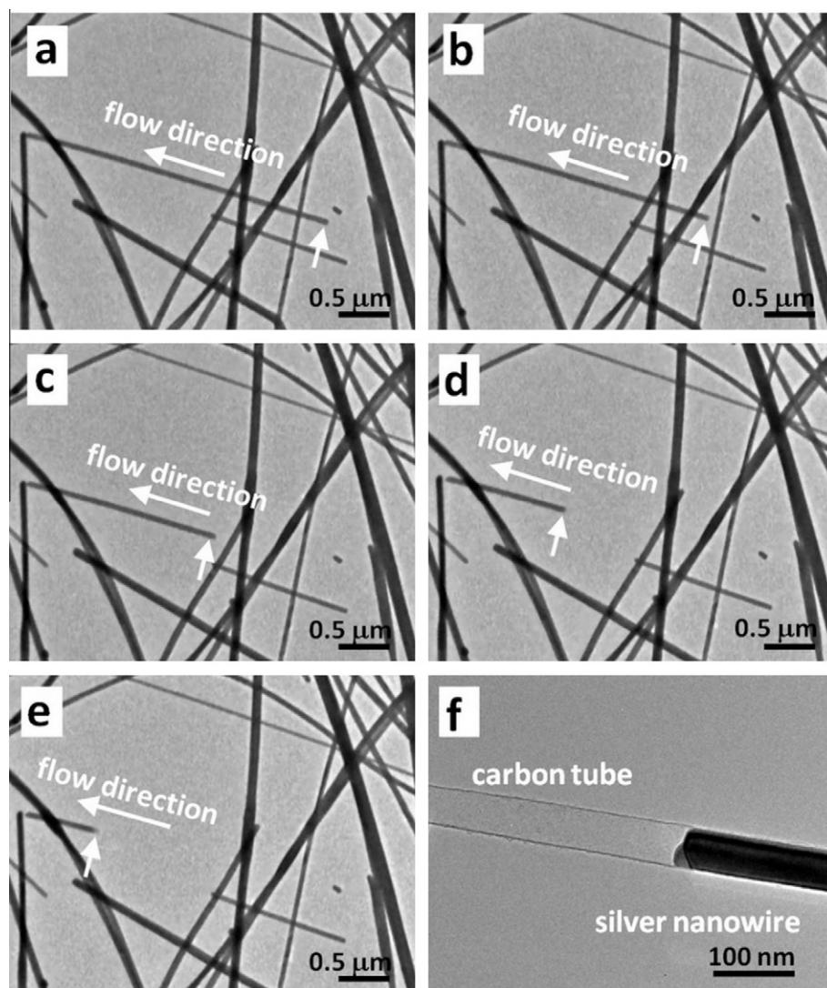
**Fig. 1 – (a–e)** A typical image sequence of extracting a molten Ag nanowire to form a CTS by heating the copper grid to 560 °C. **(f)** A snapshot of the intermediate state during extraction of the template Ag nanowire.
