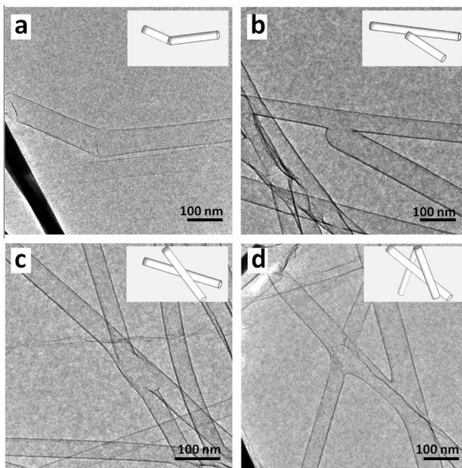
**Fig. 4 – Formation of diverse seamless CTS-based structures:** (a) a head-to-head connection, (b) a Y-shape connection, (c) a X-shape connection and (d) complex connections. Some weak points of the thin CTSs are unexpectedly damaged during extraction of the molten Ag nanowires. The insets show the schematic constructions of the Ag nanowire templates.
