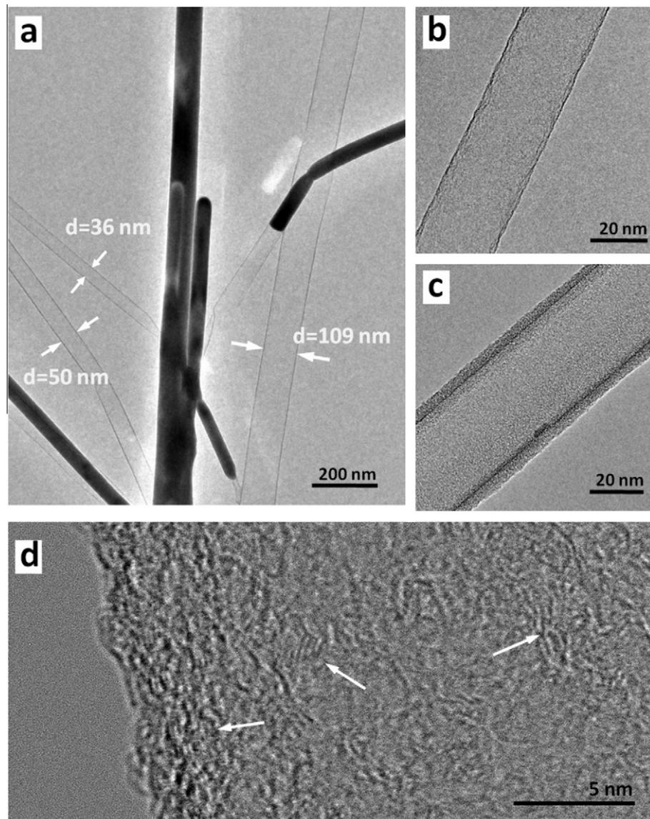
**Fig. 2 – (a)** CTSs with diverse lengths and diameters. The lengths and diameters of the CTSs are well controlled by the template Ag nanowires. **(b)** A thin-shell CTS with wall-thickness of approximately 2.3 nm. **(c)** A thick-shell CTS with wall-thickness of approximately 6.7 nm. **(d)** High resolution image of the graphitized carbon shell. The arrows indicate graphite structures after extraction of the Ag nanowires at higher temperature ( $700^\circ\text{C}$ ).
